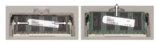
**8** Pull the memory module out of the slot.
